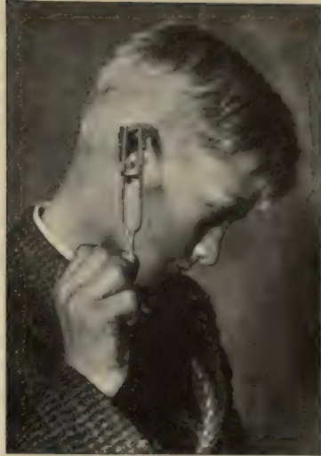
FIG. 103. When the prongs of the tuning fork are made longer or shorter, the pitch of the sound is changed.
